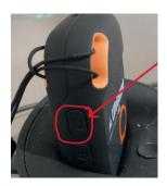
One of the first indicators is that there is no green and blue flashing lights (flashing means they are connecting to Telstra and the GPS). If the device looks like it is not charging, press the telephone symbol at the side to see if the lights start flashing and it may also vibrate. If this does not happen, or you believe there is an issue with your SmartTracker, please phone the Village Office on 6584 3515 and we will arrange for this to be sent to INS Lifeguard for repair or replacement.
